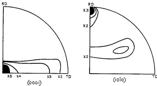
Figure 7 Pole figures of a longitudinal section of the 9.4 mm square Ti-6Al-4V bar produced by rolling in the temperature range 700 to 650°C, and subsequently annealed at 700°C.
