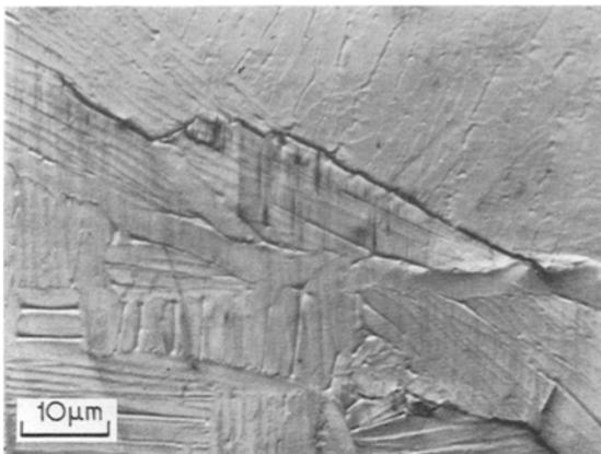
Figure 4 Interface cracking along a grain boundary on an electropolished and torsion fatigued surface of the 1.6 mm thick Ti-6Al-4V sheet.
