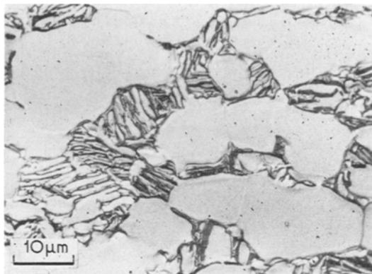
Figure 9 Microstructure of a 36 mm square Ti-6Al-4V bar produced by an 8:1 rolling reduction in the temperature range 910 to 850°C, and subsequently annealed. Etched longitudinal section.
