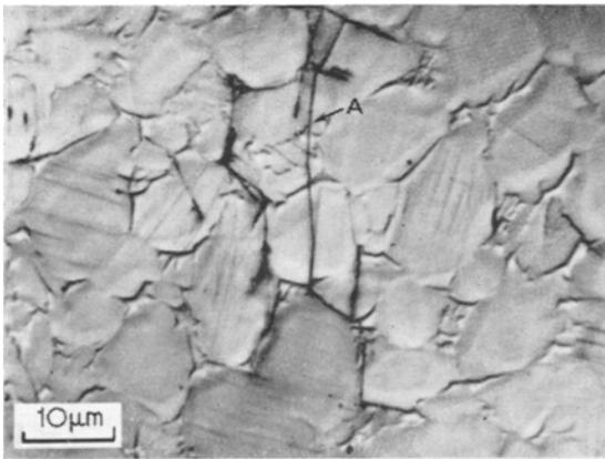
Figure 2 Transcrystalline cracking, A, on an electropolished and torsion fatigued surface of the 57 mm thick Ti-6Al-4V bar.
