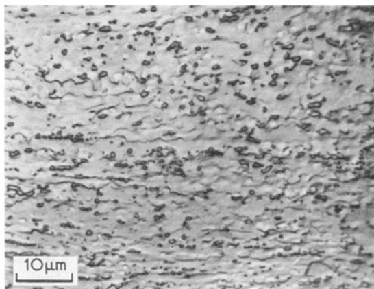
Figure 6 Microstructure of the 9.4 mm square Ti-6Al-4V bar produced by an 8:1 rolling reduction in the temperature range 700 to 650°C, and subsequently annealed at 700°C. Etched longitudinal section.
