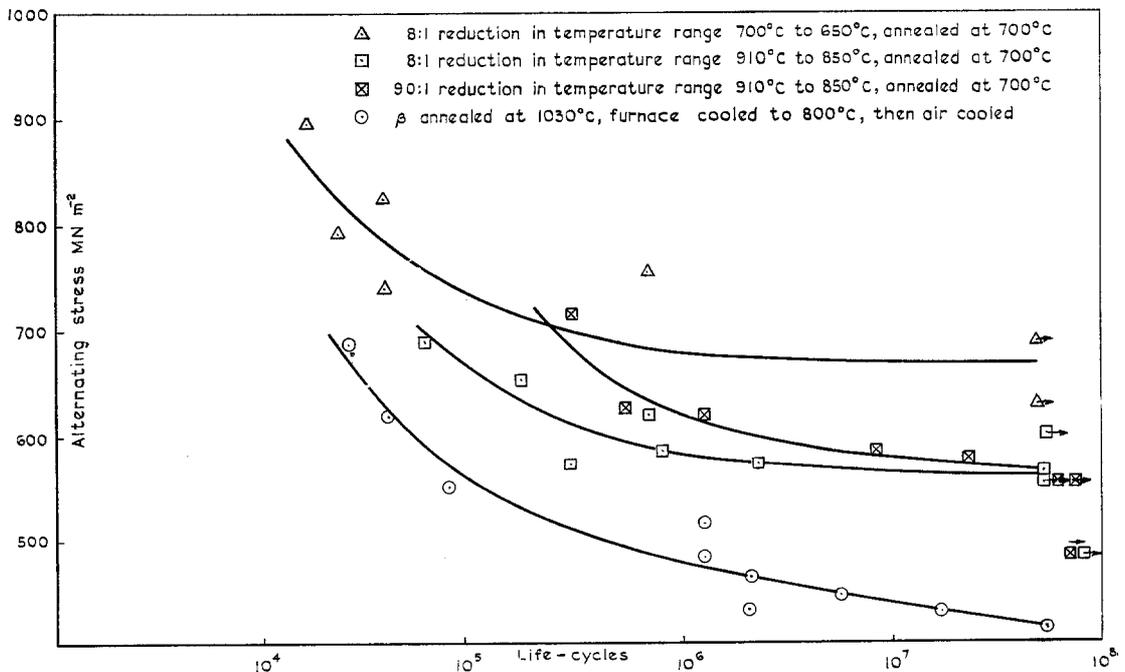
Figure 8 S-N curves for rotating cantilever fatigue tests on Ti-6Al-4V bars  $\beta$  annealed, and  $\beta$  annealed and  $\alpha + \beta$  worked at high and low temperatures in the  $\alpha + \beta$  field, and subsequently annealed.
