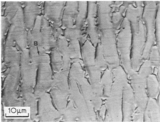
Figure 1 Crack initiation along  $\alpha/\beta$  interfaces, A, and transcrystalline deformation, B, on an electropolished and torsion fatigued surface of the 57 mm thick Ti-6Al-4V bar.
