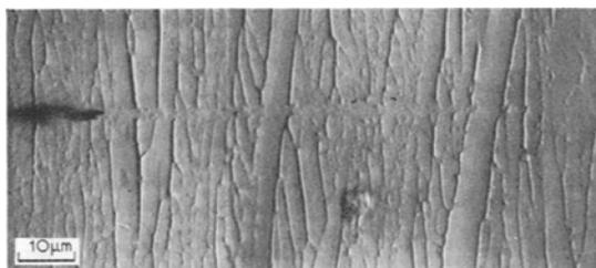
Figure 5 Damage band, A, ahead of a stage I crack tip on an electropolished and torsion fatigued surface of the 1.6 mm thick Ti-6Al-4V sheet. Specimen subsequently re-electropolished.
