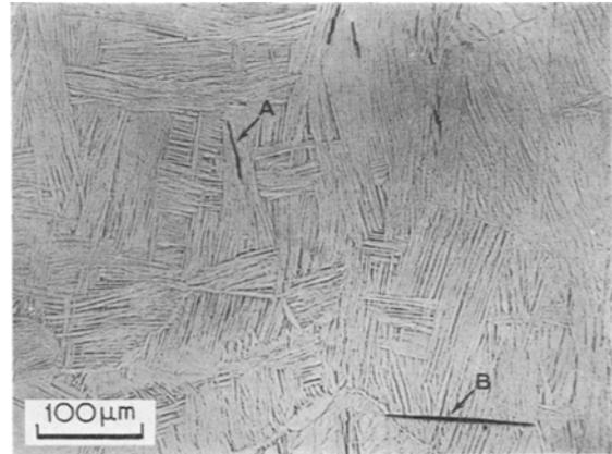
Figure 3 Crack initiation along  $\alpha/\beta$  interfaces, A, and across  $\alpha/\beta$  interfaces, B, on an electropolished and torsion fatigued surface of the 1.6 mm thick Ti-6Al-4V sheet.
