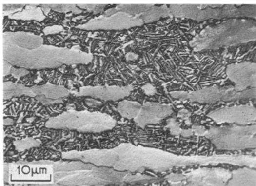
Figure 10 Microstructure of a 11 mm square Ti-6Al-4V bar produced by a 90:1 rolling reduction in the temperature range 910 to 850°C, and subsequently annealed. Etched longitudinal section.
